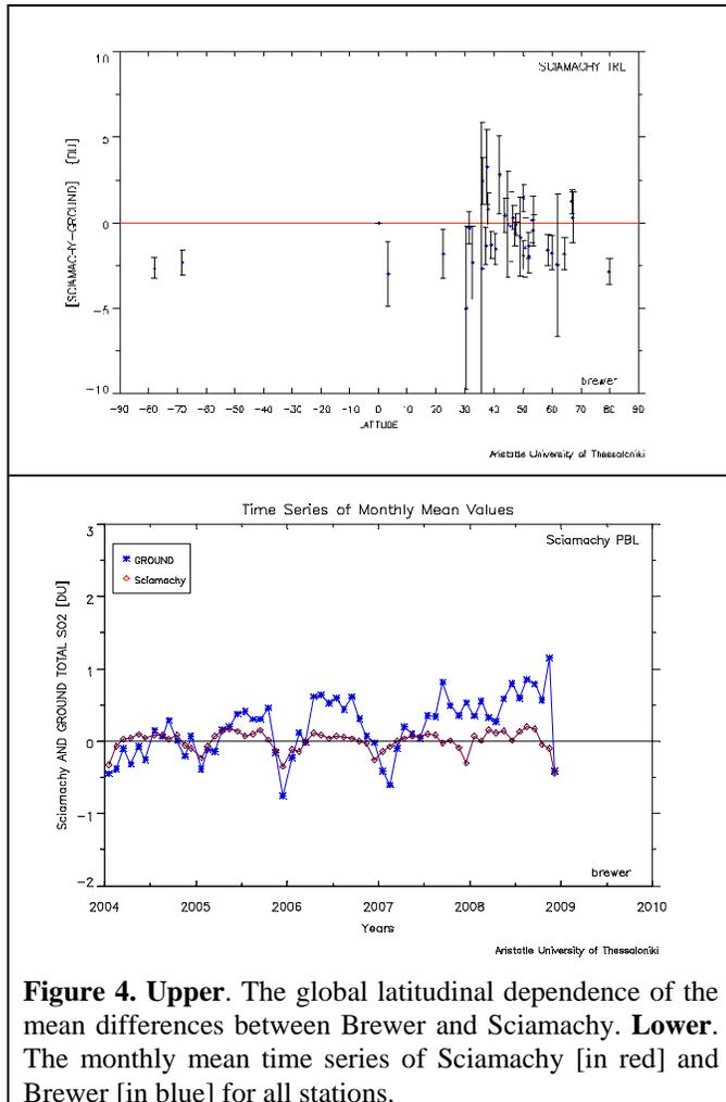
**Figure 4. Upper.** The global latitudinal dependence of the mean differences between Brewer and Sciamachy. **Lower.** The monthly mean time series of Sciamachy [in red] and Brewer [in blue] for all stations.
