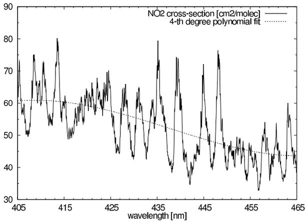
Figure 3.  $\text{NO}_2$  absorption cross section (solid; in  $\text{cm}^2/\text{molec}$ ) in the wavelength window used for  $\text{NO}_2$  retrieval, at a resolution of 0.02 nm and at room temperature, and a 4-th degree polynomial fit through it (dashed).
