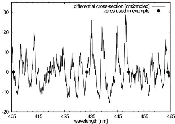
Figure 5. Differential  $\text{NO}_2$  cross section (solid line; in  $\text{cm}^2/\text{molec}$ ), the difference between the solid and dashed lines of Fig. 3, and the 5 zero points (filled circles) used for the DISMAS retrieval on the spectrum of Fig. 4.
