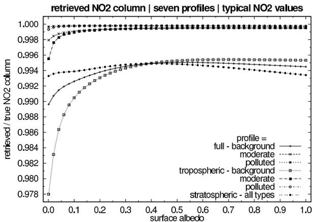
Figure 6. Bias of the retrieved  $\text{NO}_2$  column for the seven profiles, with their typical  $\text{NO}_2$  levels, as function of surface albedo. The bias is shown as retrieved divided by true  $\text{NO}_2$  column.
