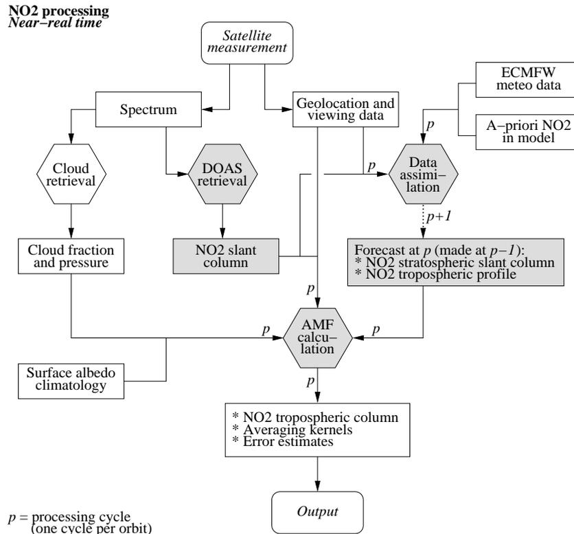
Figure 1. Schematic representation of the near-real time processing of tropospheric NO<sub>2</sub> data in the current processing system DOMINO / TM4NO2A, which applies a DOAS retrieval. The scheme shows processing cycle  $p$  in which, say, one orbit of measurements is processed. Key elements in the scheme are shaded. See Sect. 2.1 for details.
