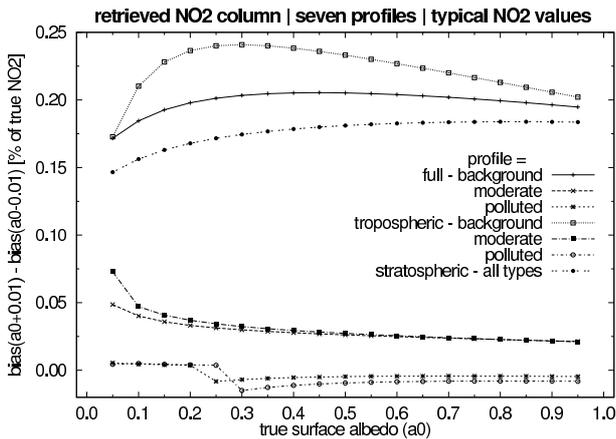
Figure 7. Difference between the  $\text{NO}_2$  retrieval biases for the assumed albedos  $a_0 + 0.01$  and  $a_0 - 0.01$ , with  $a_0$  the true albedo. The bias is a percentage of the true  $\text{NO}_2$  column for the seven profiles at their typical  $\text{NO}_2$  values.
