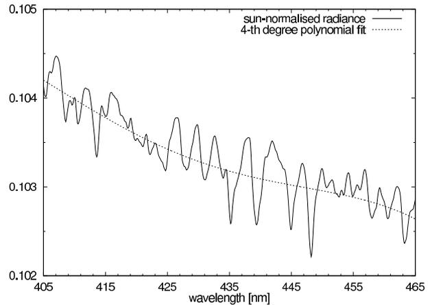
Figure 4. Example of a sun-normalised radiance (solid; dimensionless) of a simulated spectrum with a large  $\text{NO}_2$  concentration and a high surface albedo, and a 4-th degree polynomial fit through it (dashed).
