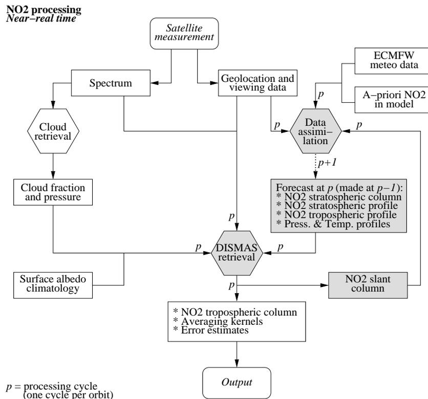
Figure 2. Schematic representation of the near-real time processing of tropospheric NO<sub>2</sub> data in the proposed processing system for TROPOMI, which applies a DISMAS retrieval. The scheme shows processing cycle  $p$  in which, say, one orbit of measurements is processed. Key elements in the scheme are shaded. See Sect. 2.2 for details.
